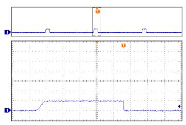
**Figure 18: Output Short Load Current** (50A/div) as a function of time when the converter attempts to turn on into a 1 m $\Omega$  short circuit. Top trace (200ms/div) is an expansion of the on-time portion of the bottom trace.
