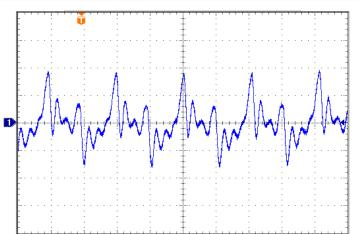
**Figure 14: Input Terminal Ripple Current**, ic, at full rated output current and nominal input voltage with  $4.7\mu$ H source impedance and  $220\mu$ F electrolytic capacitor (Ch.1 500mA/div). (See Figure 13).
