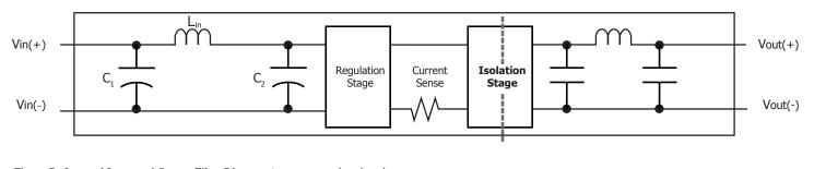
Figure D: Internal Input and Output Filter Diagram (component values listed in Electrical Characteristics section).
