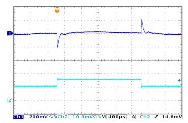
Figure 12: Output Voltage Response to Step-Change in Load Current (50%-75%-50% of lout(max):  $dI/dt = 5A/\mu s$ ). Load cap:  $330\mu F$  electrolytic output capacitance. Top trace: Vout (200mV/div). Bottom trace: lout (20A/div).
