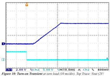
*Figure 10: Turn-on Transient* at zero load (10 ms/div). Top Trace: Vout (2V/ div). Bottom Trace: ON/OFF input (5V/div)
