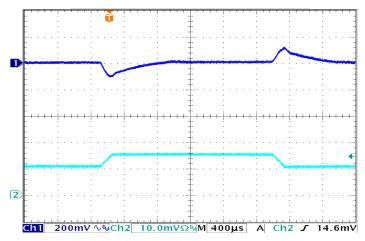
Figure 11: Output Voltage Response to Step-Change in Load Current (50%-75%-50% of Iout(max);  $dI/dt = 0.1A/\mu s$ ). Load cap:  $100\mu F$  electrolytic output capacitance. Top trace: Vout (200mV/div). Bottom trace: Iout (20A/div).
