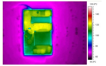
*Figure 8: Thermal Image* of converter at 32.7 amp load current (164W) with 55°C air flowing at the rate of 200 LFM. Air is flowing across the converter from output to input (nominal input voltage).
