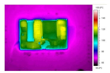
Figure 6: Thermal Image of converter at 34.0 amp load current (170W) with 55°C air flowing at the rate of 200 LFM. Air is flowing from pin 3 to pin 1 (nominal input voltage).
