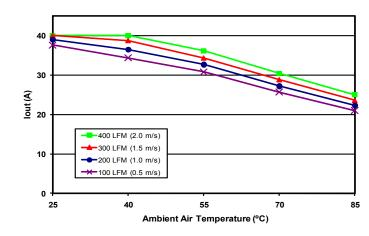
Figure 7: Thermal Derating (max output current vs. ambient air temperature) for airflow rates of 100 LFM through 400 LFM with air flowing lenghtwise from output to input (nominal input voltage).
