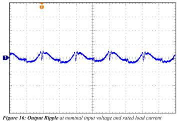
(50 mV/div). Load capacitance: one  $1.0\mu F$  ceramic capacitor and one  $100\mu F$ electrolytic capacitor. Bandwidth: 20 MHz. (See Figure 13).
