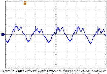
at nominal input voltage and rated load current (10 mA/div). (See Figure 13).
